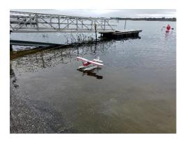
used. The Maule M-7 comes with floats that include a servo-operated water rudder. Horizon's Timber airplane line, less the Timber X, each include a set of floats with dual water rudders hooked to the aircraft rudder by fishing line. Those floats will also fit the non-float equipped Timber X.
